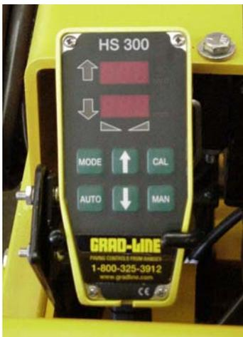
1. Place the handset into the cradle at the operator's station. Route cable over the resting bolt.
